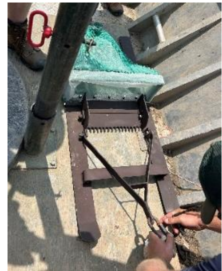
The Ponar (Top) and the Benthic Sled (Bottom) in use on the Open River
